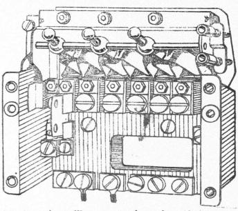
The three illustrations show the switch-board, starter switch, and cut-out as embodied in the C.A.V. electrical equipment which is fitted to the 1925 four-cylinder 28/60 h.p. Vauxhall, a wiring diagram of which is on the previous page.
