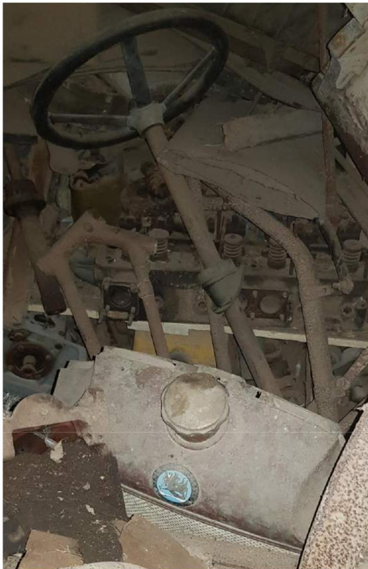
23-60 radiator, head with steering wheel and column
