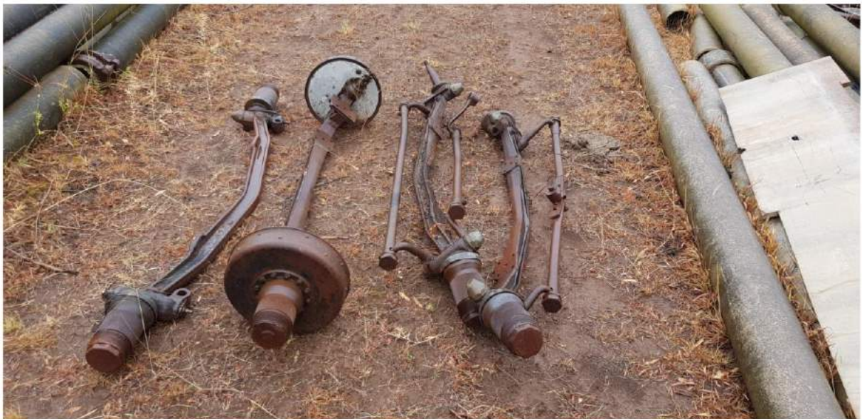
Three unbraked 23-60 front axles and one braked axle
