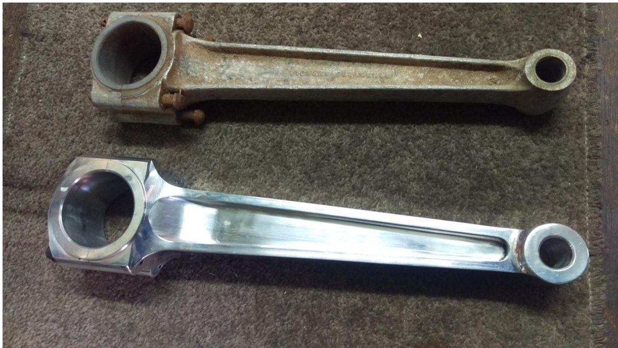
New OE – OD rod made by Sainty Engineering with original rod
